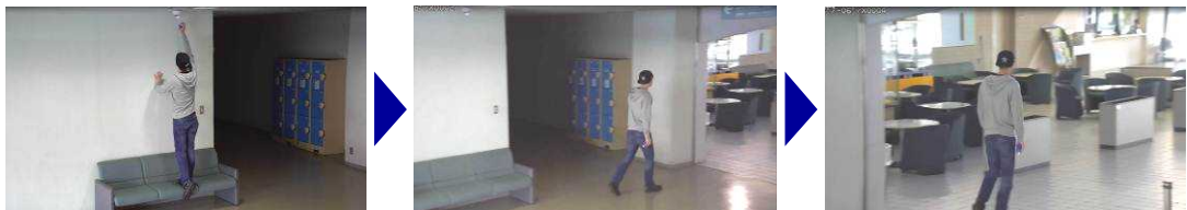
Figure 12: Advanced Auto Tracking and Scene Change Detection (i-VMD). In this example, when a camera was tampered, another PTZ camera started tracking by Panasonic inter-camera notification protocol from the tampered camera.
